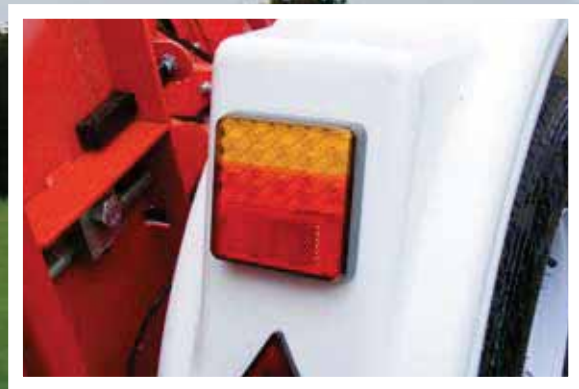
Multi-voltage LED road lighting.
