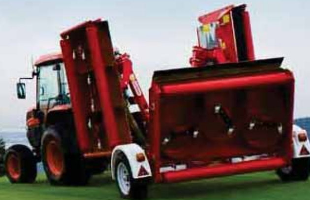
Moving between locations is a safe and easy exercise. Decks are hydraulically lifted and automatically locked into place for transport mode.
