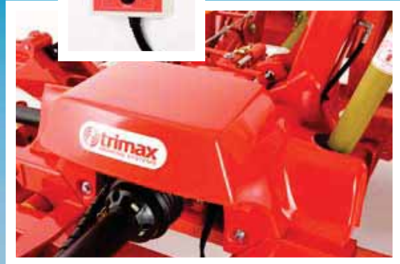
Moulded cover for electro-hydraulic controls (Elite only).
