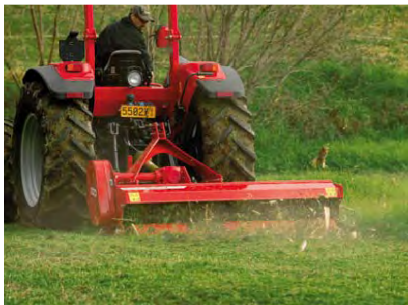
Shreds prunings up to 75mm (3") in diameter.
